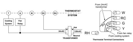
Figure 6. Typical Wiring Diagram for Cool Only, 3-Wire, Single Transformer Systems
